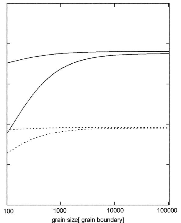
**Fig. 5** Grain size dependence of the bulk modulus (upper and lower bounds, solid lines) and shear modulus (upper and lower bounds, dotted lines) for parameters given in the text. The length scale is given in units of the interfacial thickness which can be estimated to be 1 nm. Interfacial softening occurs in this case for grain sizes smaller than some 5  $\mu\text{m}$
