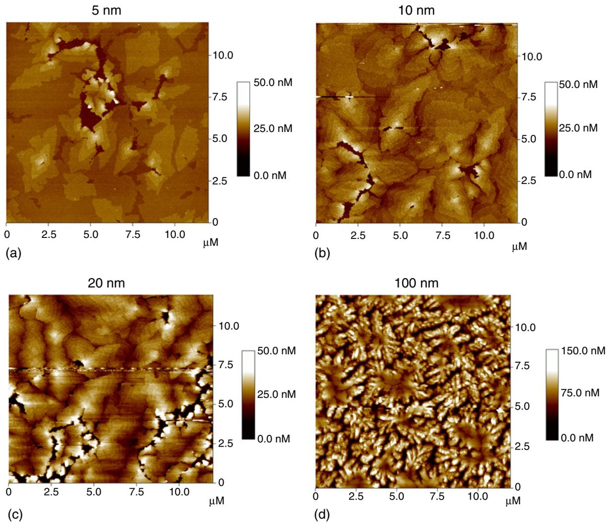
**Figure 2.** AFM images of the conduction channel. The channel morphology changes as the film thickness is increased. The best film structure is in the ultrathin transistor while the worst (dendritic) is in the 100 nm thick pentacene film where the bulk imperfections determine the film growth process.
