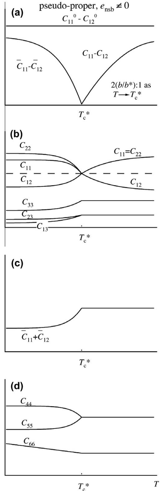
**Fig. 4.** Schematic form of elastic constant variations expected for a pseudoproper ferroelastic tetragonal  $\leftrightarrow$  orthorhombic phase transition. From Fig. 9 of Carpenter and Salje (1998)
