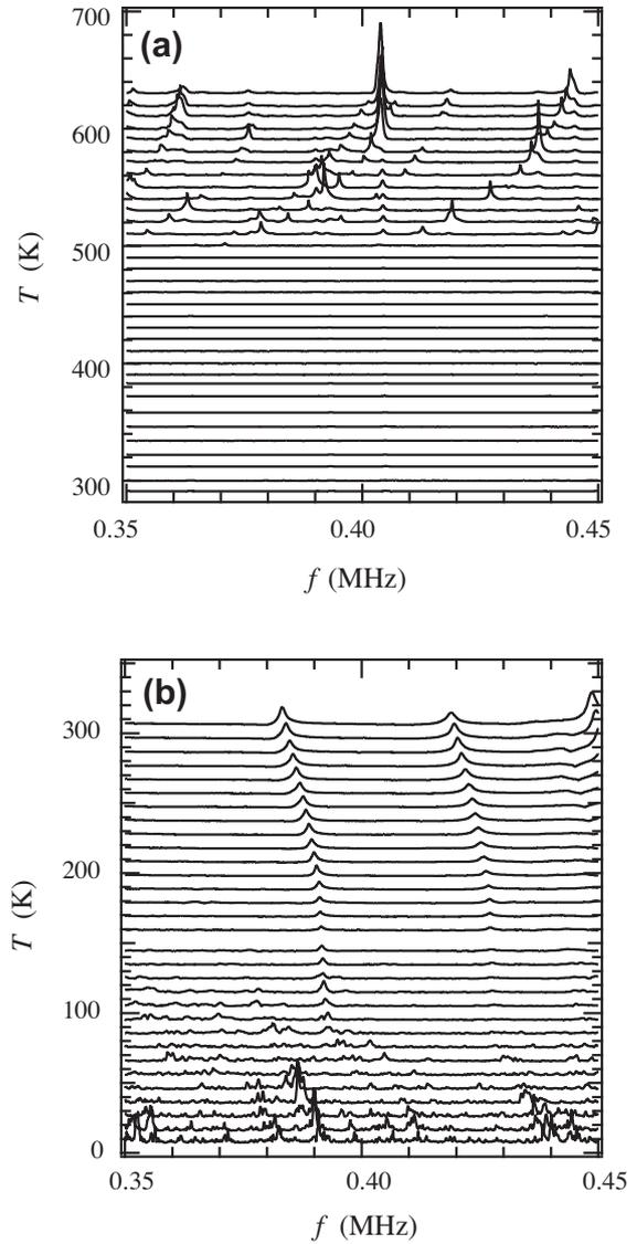
Fig. 1. Stacks of RUS scans for CaCl<sub>2</sub>. (a) High temperatures. Regularly spaced background peaks are due to the alumina buffer rods. (b) Low temperatures. The background peaks at very low temperatures are noise from somewhere in the sample holder.
