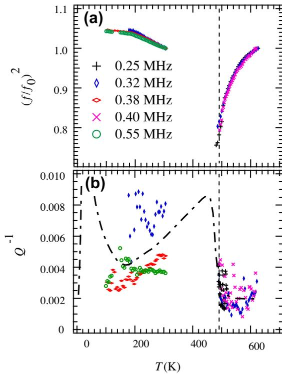
**Fig. 2.** Temperature dependencies of normalised square of frequency  $(f/f_0)^2$  and inverse quality factor  $Q^{-1}$  of  $\text{CaCl}_2$  determined by RUS. The dashed line is the transition temperature 491 K. The dash-dotted curve shows the pattern of loss behaviour typical of that due to ferroelastic twin wall mobility below the transition point followed by pinning at some lower temperatures.
