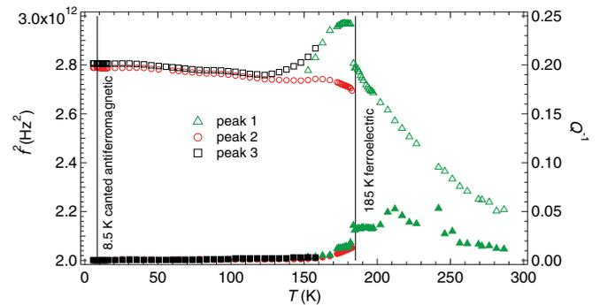
FIG. 7. (Color online) Variation with temperature of  $f^2$  (open symbols) and  $Q^{-1}$  (closed symbols) for peaks labeled in Fig. 6. Phase transitions are displayed as black solid lines. Data were scaled so as to overlap at  $\sim 10 \text{ K}$ .
