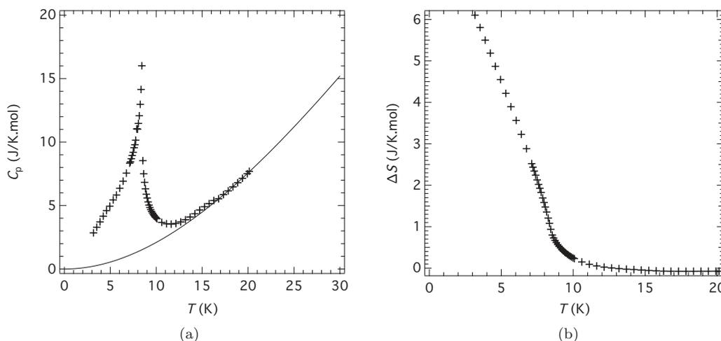
FIG. 8. (a) Fit of Eq. (3) to heat capacity data from Jain *et al.*<sup>32</sup> in the temperature region 0–30 K, and (b) the excess entropy associated with magnetic ordering in DMAMnF.
