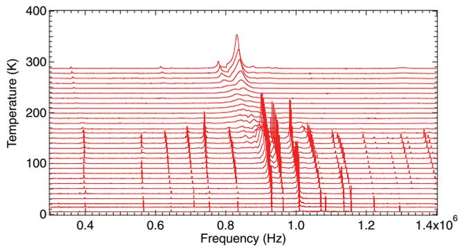
FIG. 2. (Color online) Selected RUS spectra of DMACoF displayed as a stack plot. The y axis should be the amplitude in volts, but the spectra have been offset in proportion to the temperature at which they were collected and the axis is therefore labeled as temperature. Note the disappearance of most peaks above  $\sim 170$  K.
