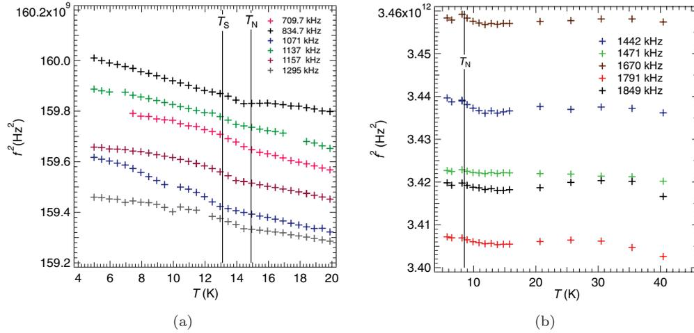
FIG. 5. (Color online) (a) Enlargement of low temperature variations of  $f^2$  for several peaks of DMACoF scaled to appear in the range  $(159.2\text{--}160.2) \times 10^9 \text{ Hz}^2$ . (b) Low temperature variation of  $f^2$  for several peaks of DMAMnF scaled to appear in the range  $(340\text{--}346) \times 10^{12} \text{ Hz}^2$ . Magnetic transition temperatures are displayed as solid black lines. Peaks are labelled with their frequency values at  $\sim 5 \text{ K}$ .
