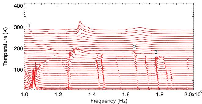
FIG. 6. (Color online) Stack plot of RUS spectra for DMAMnF, with peaks analyzed in Fig. 7 labeled, and spectra offset on the y axis in proportion to the temperature at which they were collected. Some spectra are omitted for clarity.
