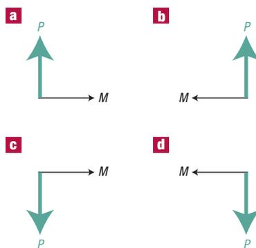
**Figure 2** The four degrees of multiferroic order. **a–d**, Electric polarization  $P$  and magnetization  $M$  can assume four non-collinear states in a multiferroic crystal. In this schematic with arbitrary magnitudes, the directions are in real space. For some materials the spins and polarizations are highly correlated<sup>10,11</sup>, so that only pairs **a** and **d** or alternatively **b** and **c** are readily accessible.
