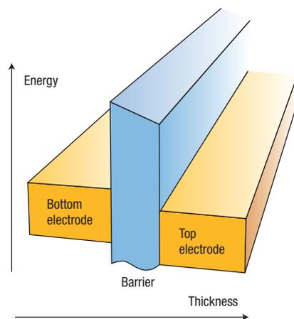
**Figure 1** Schematic of a tunnel junction. Electrons tunnel from the bottom electrode through the barrier into the top electrode.
